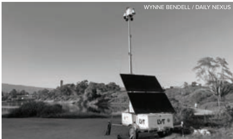
The 180-degree cameras are part of mobile security units, which also include floodlights, spotlights and speakers.
